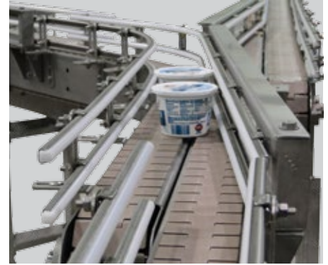
Stainless Steel Modular Table Top Conveyor System with Plastic Chain, Double High Adjustable Rail UHMW Side Guides and Manual Divert Arm with Adjustable Rail UHMW Side Guides
